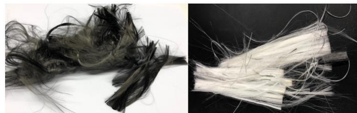
Figure 2: recovered fibres after the burning
