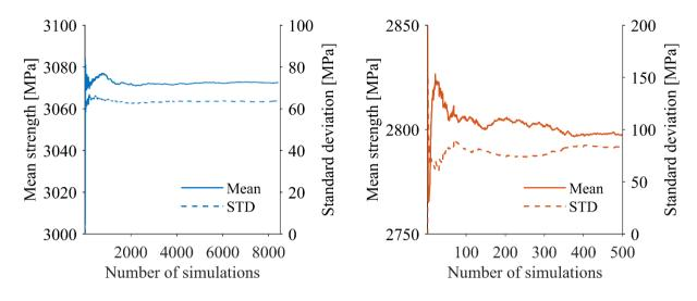
Figure 4 Convergence of the mean and standard deviation of fibre break model results for  $V_f = 0.5$ .
