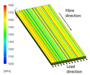
**Figure 1** Probability distributions of bundle strengths for different  $V_f$  calculated with the fibre break model.
