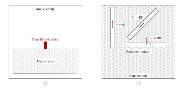
Figure 1. Specimen manufacturing: (a) initial material placement before compression moulding, and (b) moulded plate after compression moulding. Red arrows indicate, in both figures, the main flow direction.
