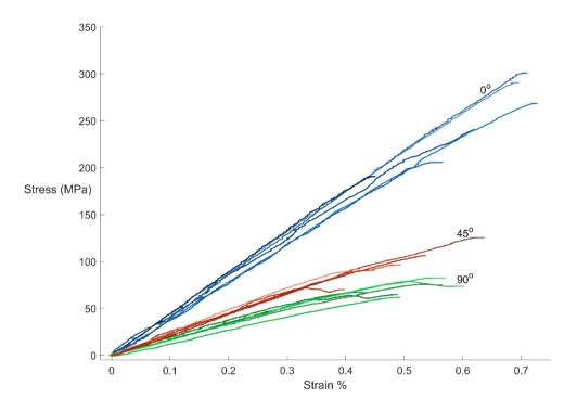
Figure 2. Stress-strain curves of specimens at different prevalent orientation
